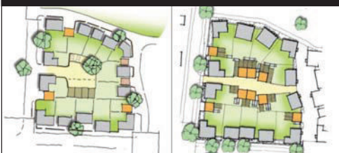
Figure 10 Trumpington Meadows, indicative arrangement of off-plot car parking showing rear court (left) and mews arrangement (right)
